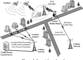
Figure 1. Smartphone-based Traffic Information System
